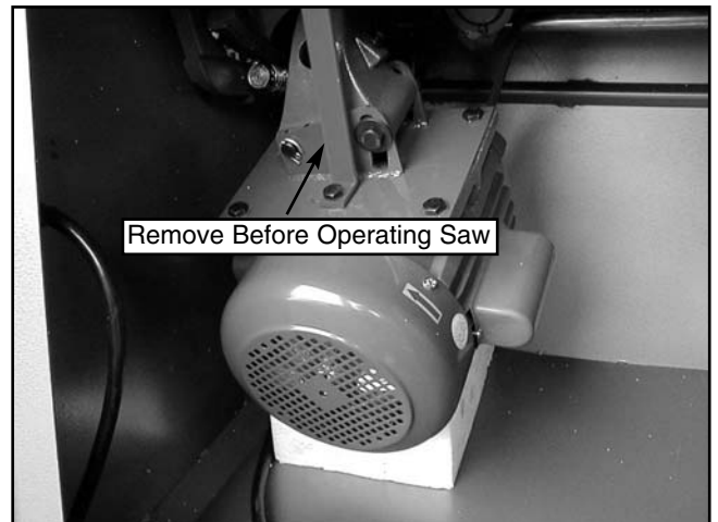
Figure 11. Remove motor bracket.
